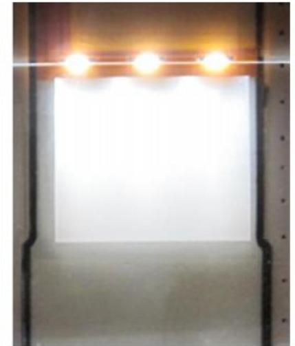
**Fig. 1.** Flexible Ni-mold consisting one 28 × 28 mm size backlight device. Mold thickness is 300 μm.
